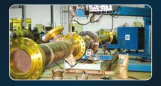
Alfa Pipiline Products Cladding Division is equipped with fully automated system for weld cladding pipeline components and oil field equipments. We can handle cladding from Ø 2" to Ø 56" components. We have the right experience to provide cost effective solutions for the Oil & Gas Industries.
