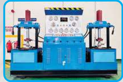
Pressure Testing upto 21 Valves Simultaneously
